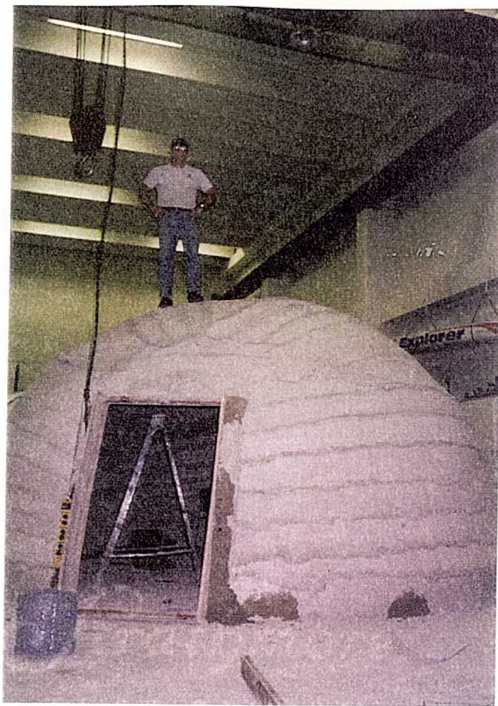
Figure 25. Finished 1/2" thick dome with 190 lb. point load on top.
