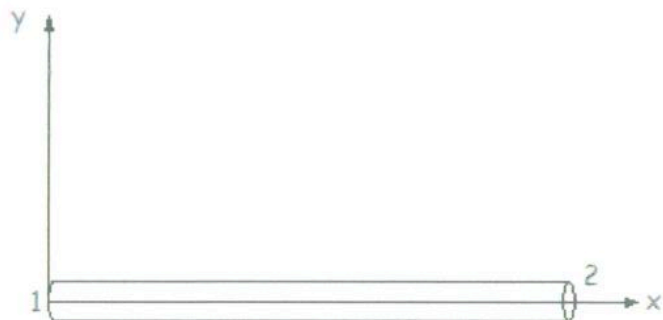
(a) Simple line element typically used to represent a bar or beam element
