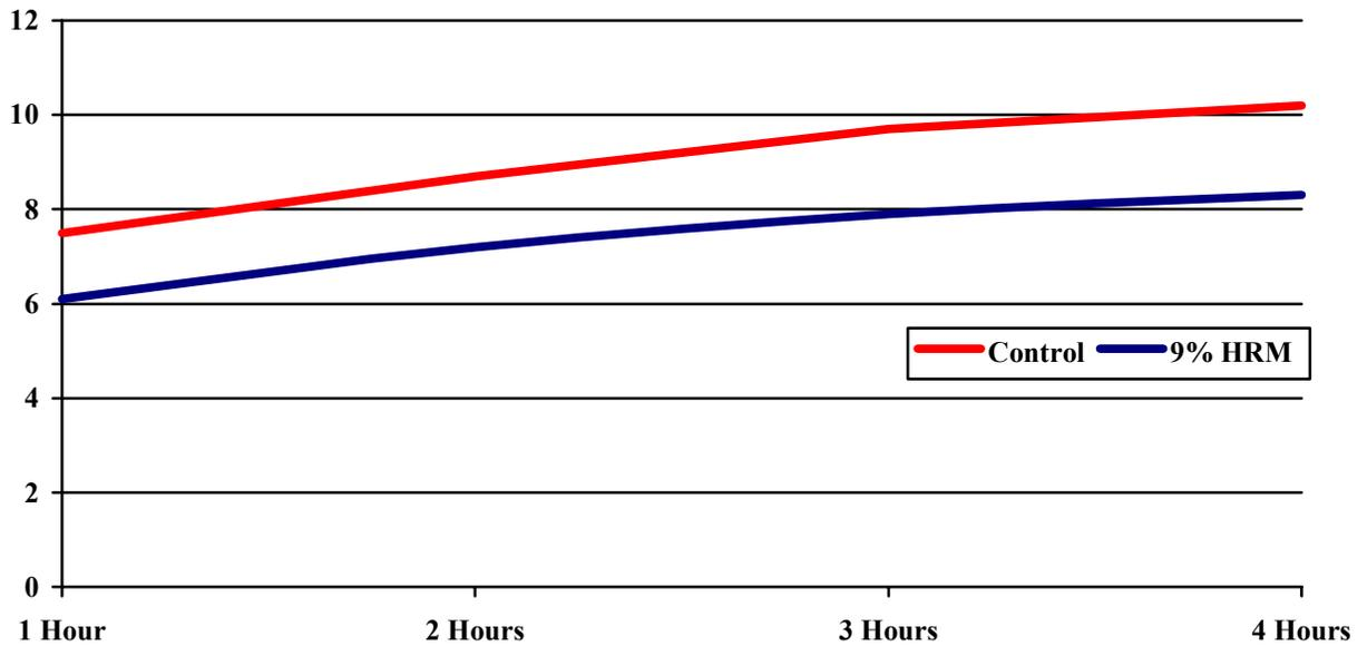
Figure 4. Effect of HRM on water absorption in a grout formulation.
