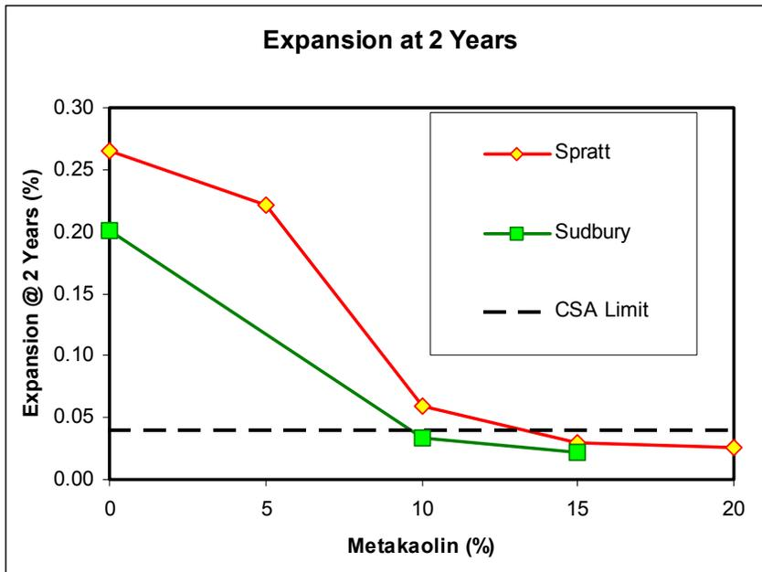
Figure 5. Effect of HRM on ASR.
