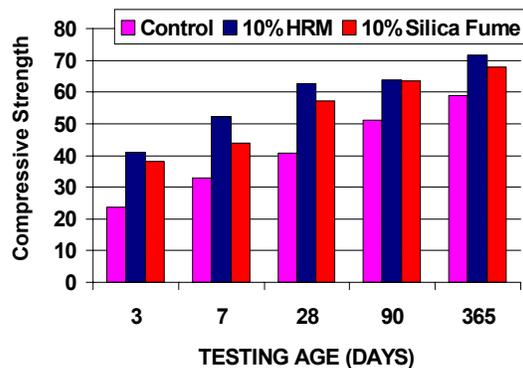
Figure 1. Comparison of compressive strength with time for HRM and SF with the mixture design in Table 1.
