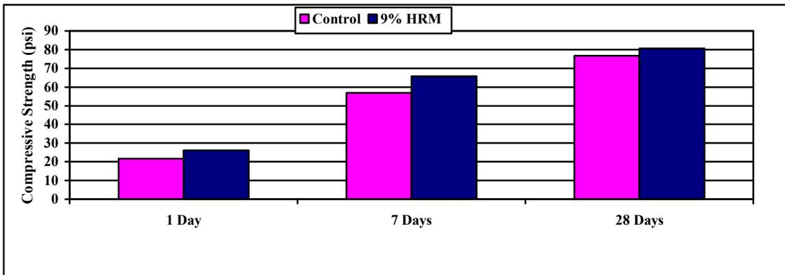
Figure 3. Compressive strength improvement in a grout formulation by replacement of cement with HRM.
