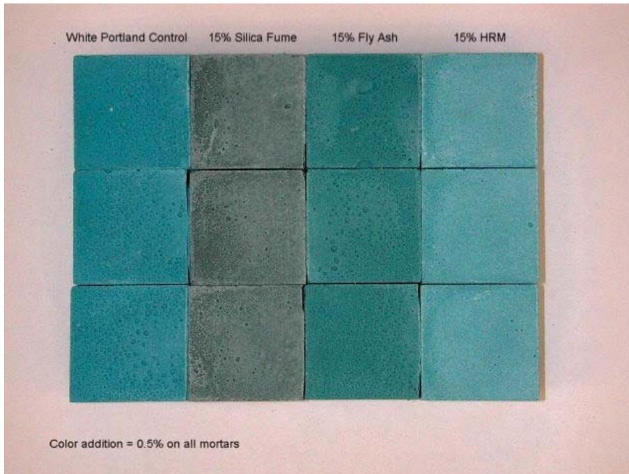
Figure 7. Addition of pigment (bright blue in this case) to WPC can only be matched by HRM and not SF or FA.
