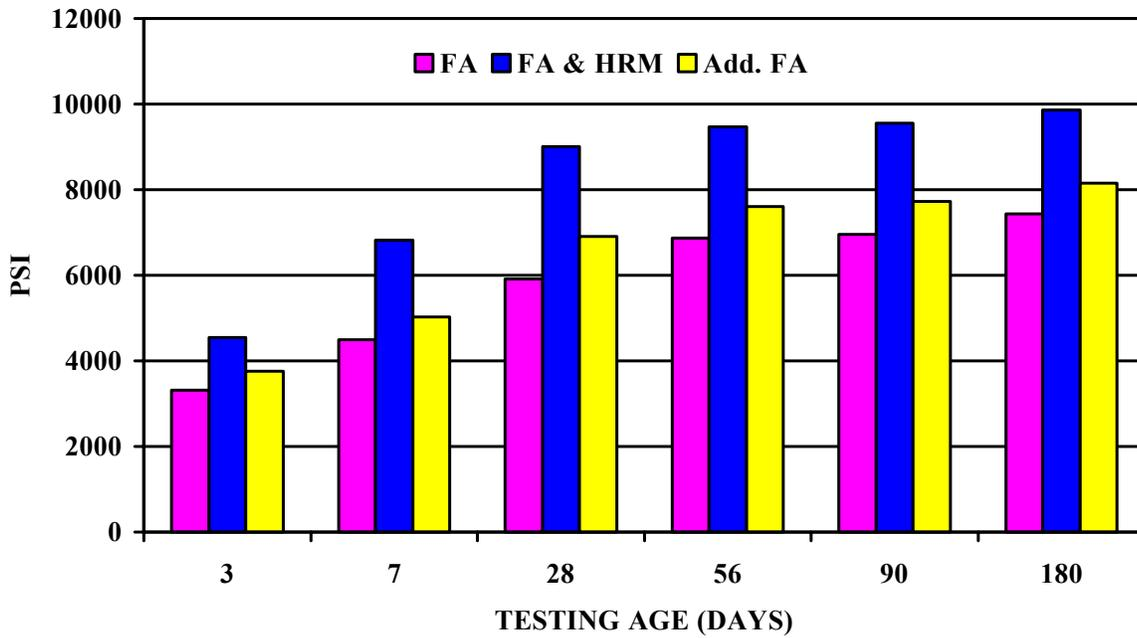
Figure 8. Increase in compressive strength with HRM compared to FA as well as additional FA.
