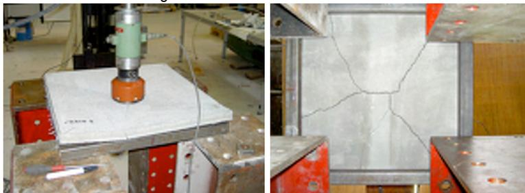
Figure 10.20: Crack develop on upper side of plate
