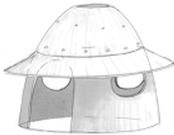
Figure 7.15: An example of a dome taking several of the matching building responses into account. However the hole in the roof should preferably be shaded by an elevated cover
