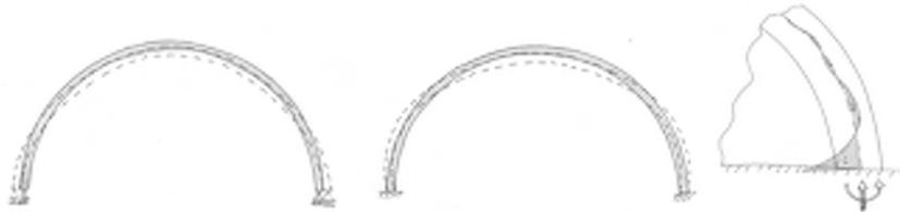
Figure 8.1: The connection to the foundation is rigid and prevents the shell from deforming as in most left sketch. Consequently the shell deforms as in the middle sketch. The moments that stem from this edge disturbance are shown in the sketch on the right.
