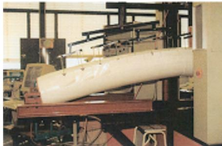
Figure 11.23: Experiment of Frank Braam; a pneumatic tube loaded by a (roughly) uniform distributed load pulling on the upper side of the beam [Braam, 2000]
