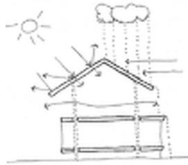
Figure 7.4: The roof acting as a parasol, protecting the inner spaces from sun and rain as well as maximizing ventilation below the roof [Hyde, 2000]
