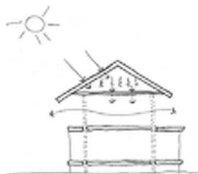
Figure 7.6: Ventilation is crucial to removing heat in an attic roof, otherwise back radiation from the roof surface heats the attic air which is radiated via the ceiling to the internal air below [Hyde, 2000]
