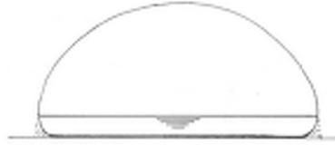
Figure 11.2: Closed formwork loaded with water, to reduce deformations at least 22 000 liter water is needed. Deformations at the sides are compensated with i.e. adobe before the ferrocement or concrete is applied.
