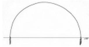
Figure 9.7: Anchoring uplifting forces with groundanchors
