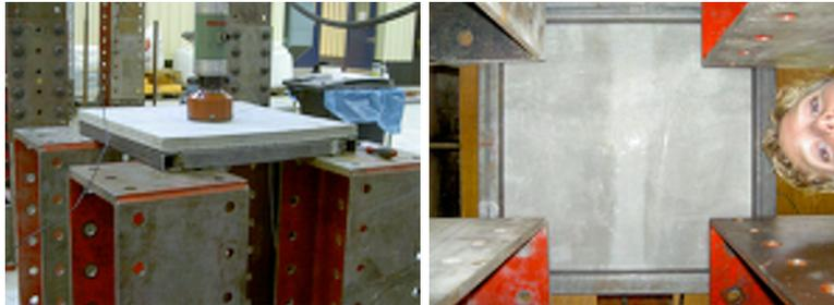
Figure 10.18: First cracks develop
