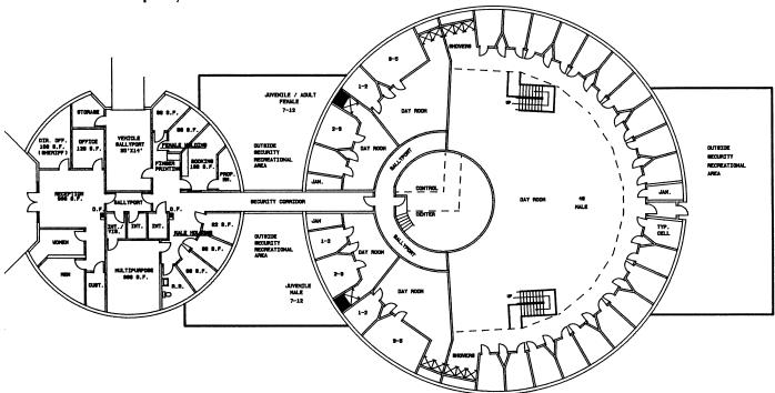
Preliminary Concept 2 72' Diameter Administration Dome Two 50' Diameter and One 92' Diameter Security Domes for Juveniles 68 to 76+ Inmate Capacity
