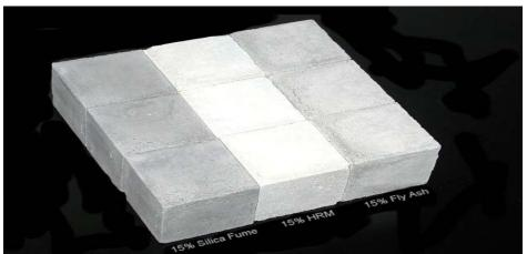
Figure 6. Mortars containing WPC with 15% SF, HRM and FA
