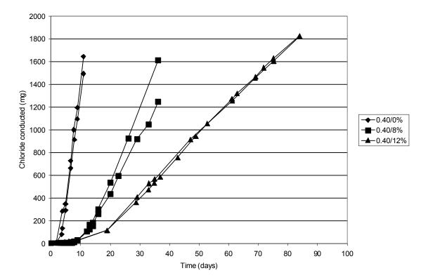
Figure 2. Effect of HRM addition on Chloride Migration
