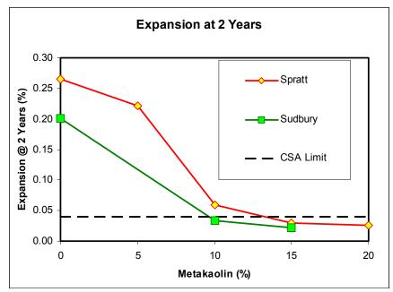
Figure 5.Effect of HRM on ASR.
