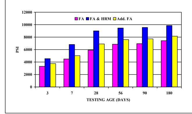
Figure 8. Increase in compressive strength with HRM compared to FA as well as additional FA.
