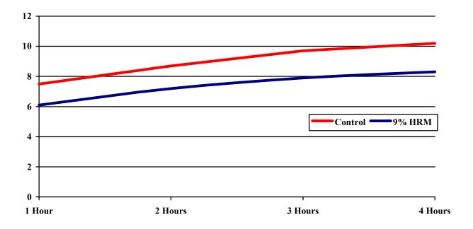
Figure 4. Effect of HRM on water absorption in a grout formulation.
