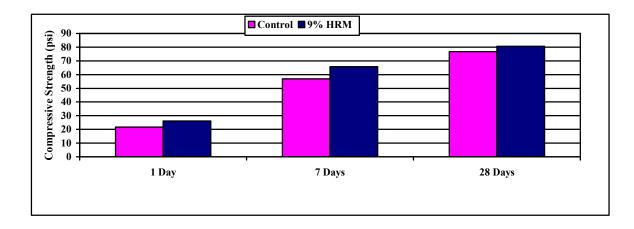
Figure 3. Compressive strength improvement in a grout formulation by replacement of cement with HRM.
